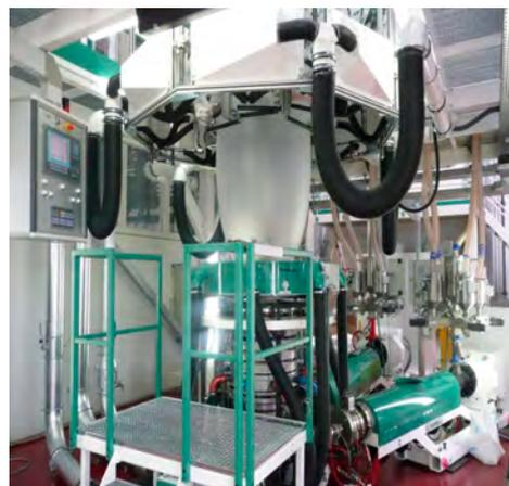
3 Layer Co-Extrusion of Bio-Flex<sup>®</sup>
