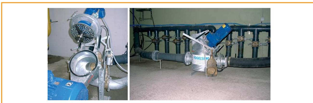
Figure 3.8: In-pipe substrate comminution (perforated-plate comminutor) [Hugo Vogelsang Maschinenbau GmbH]
