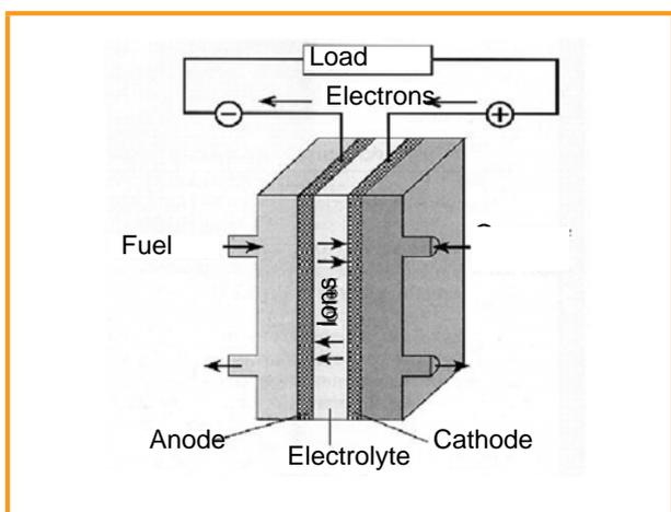
Figure 6.12: Operating principle of a fuel cell [vTI]
