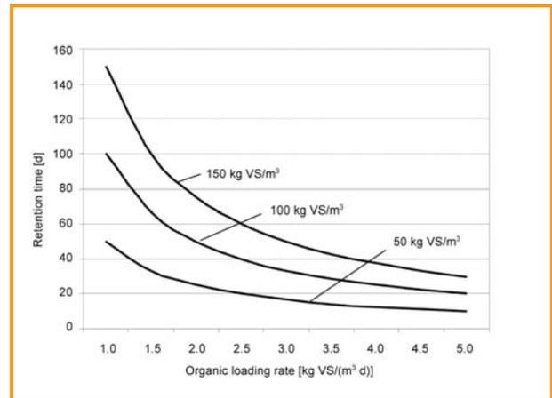
Figure 2.2: Correlation between organic loading rate and hydraulic retention time for various substrate concentrations
