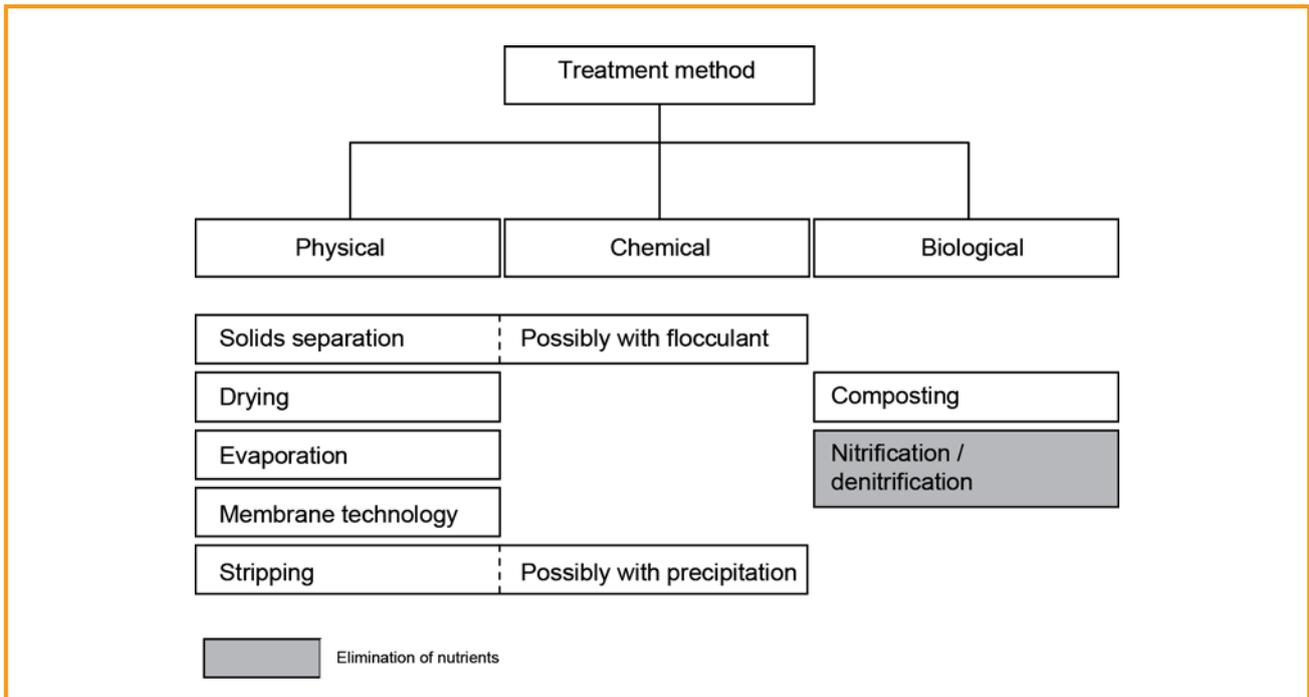
Figure 10.7: Classification of treatment processes by type
