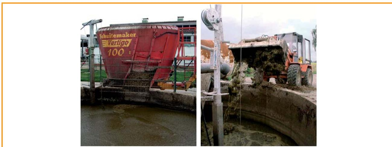
Figure 3.14: Pre-digester or receiving pit in feeding [Paterson, FNR; Hugo Vogelsang Maschinenbau GmbH]
