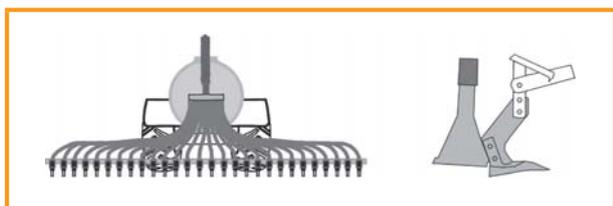
Figure 10.3: Trailing shoe applicator
