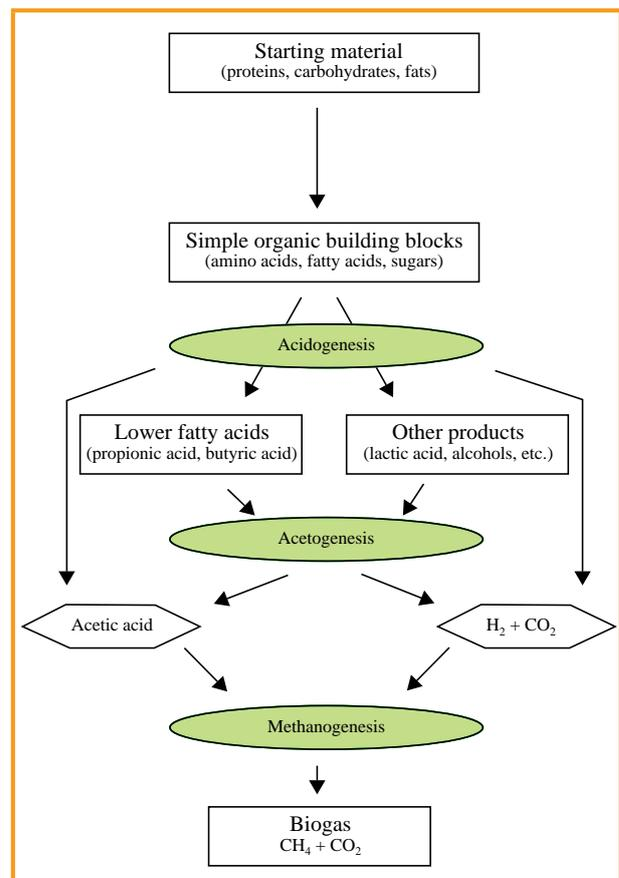
Figure 2.1: Schematic representation of anaerobic decomposition
