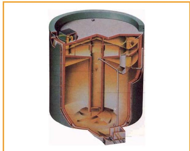
Figure 3.27: Two-chamber digester [ENTEC Environment Technology Umwelttechnik GmbH]
