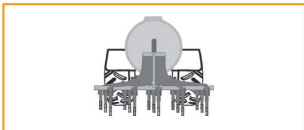
Figure 10.5: Manure injector
